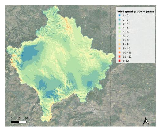
Figure 2-5 Wind speed at 100 m a.g.l. in Kosovo (source: <u>https://globalwindatlas.info/</u>)
