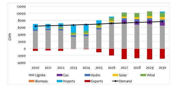
Figure 5-64 Electricity generation per technology in S5.2 scenario
