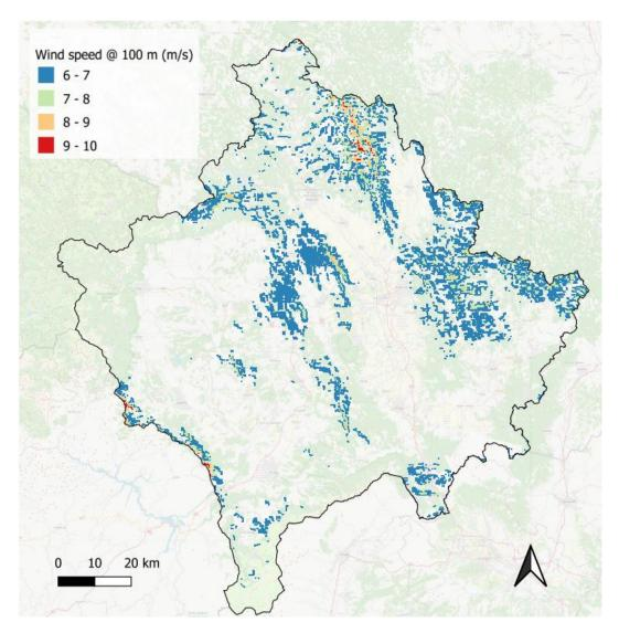
Figure 2-14 Wind speed in the range from 6 m/s to 10 m/s outside exclusion zones
