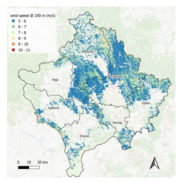
Figure 2-16 Wind speed in the range from 5 m/s to 11 m/s outside of exclusion zones
