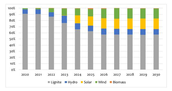
Figure 5-56 Generation shares per technology in Base without TPP Kosova e Re scenario with utility-scale PV candidate at depleted mine
