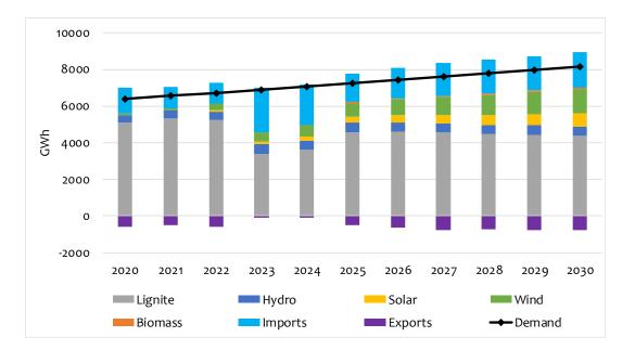
Figure 5-28 Electricity generation per technology in High with TPP Kosova e Re scenario
