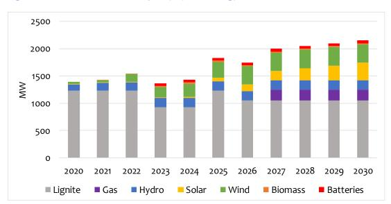
Figure 5-61 Total installed capacity by technology in S5.3 scenario
