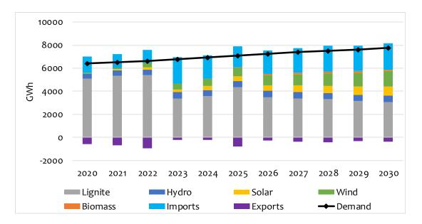
Figure 5-18 Electricity generation per technology in BaU without TPP Kosova e Re scenario
