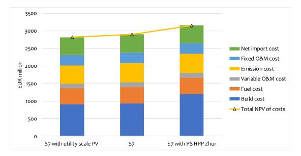
Comparison of NPV of total costs in Base without TPP Kosova e Re with the two scenarios analysed (large-scale utility PV and PS HPP Zhur) is shown in the following figure.
