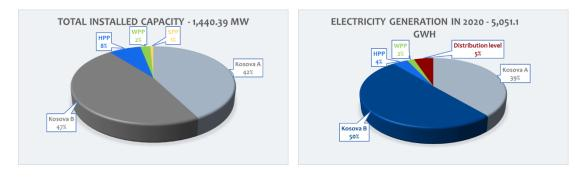
Figure 0-1 Power plants capacity and expected electricity generation in 2020
