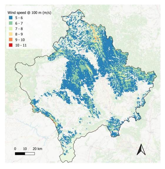
Figure 2-13 Wind speed in the range from 5 m/s to 11 m/s outside exclusion zones
